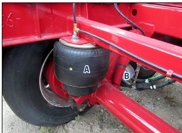
A - Air Bag B - Shock Absorber
