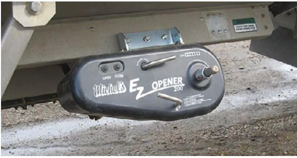
Figure 16 – Michel's Electric Chute Gate Drive
