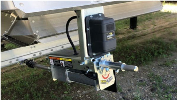
Figure 17 – Shur-Co Electric Chute Gate Drive
