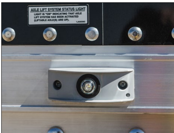
Figure 24 – Axle Lift System Decal and Light
