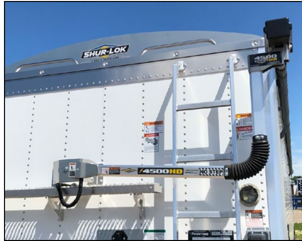
Figure 27 – Electric Tarp Drive
