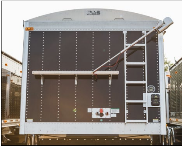
Figure 25 – Electric Tarp Drive
