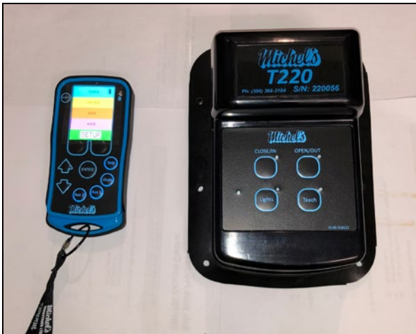
Figure 26 – Tarp Control Box
