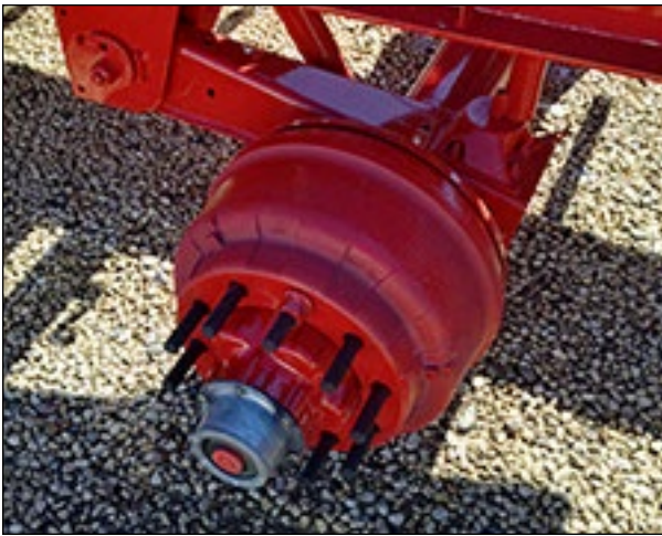
Figure 42 – Drum Brake Package
