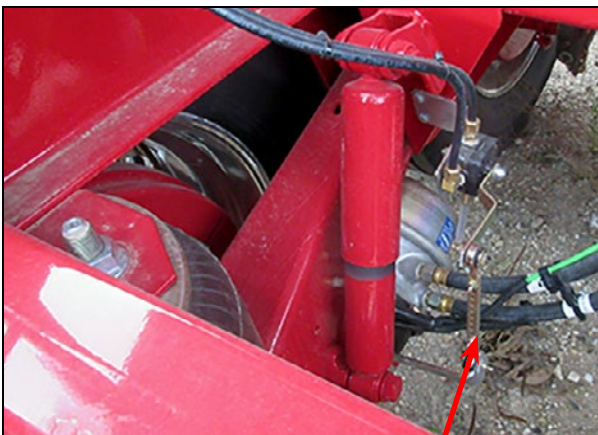
Figure 32 – Ride Height Mechanism
