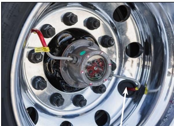
Figure 19 – Tire Inflation Hoses
