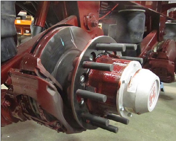
Figure 43 – Disk Brake Package
