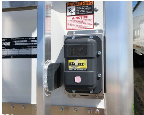
Figure 28 – Tarp Control Box
